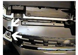
**1.** Remove metric bolt with the 10MM socket and one phillips push pin on top edge of grill, both sides.
