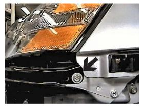
8. Remove metric bolt from lower side of head light assembly using the 10MM socket, both sides.
