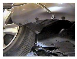
**4.** Forward of front tires are four push pins to remove from lower edge of fascia, both sides.
